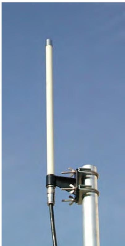
This antenna is a narrow band design for secondary radar ( IFF ) from 1070 to 1110 MHz. Due to the omnidirectional characteristic and the medium gain the reception is good in any direction, also up. Cable not included.
